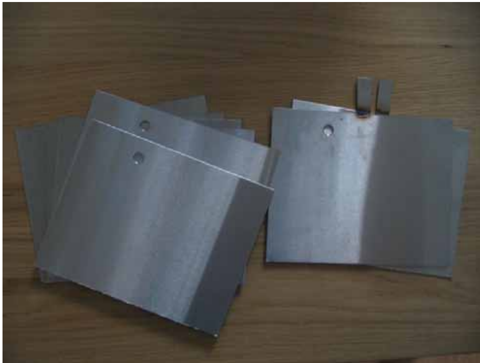
Figure 2. Stainless steel electrolyzer plates (8 total)
