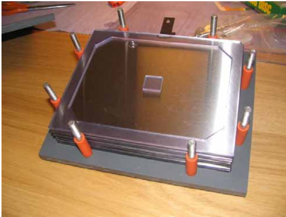
Figure 6. Partly assembled cell stack
