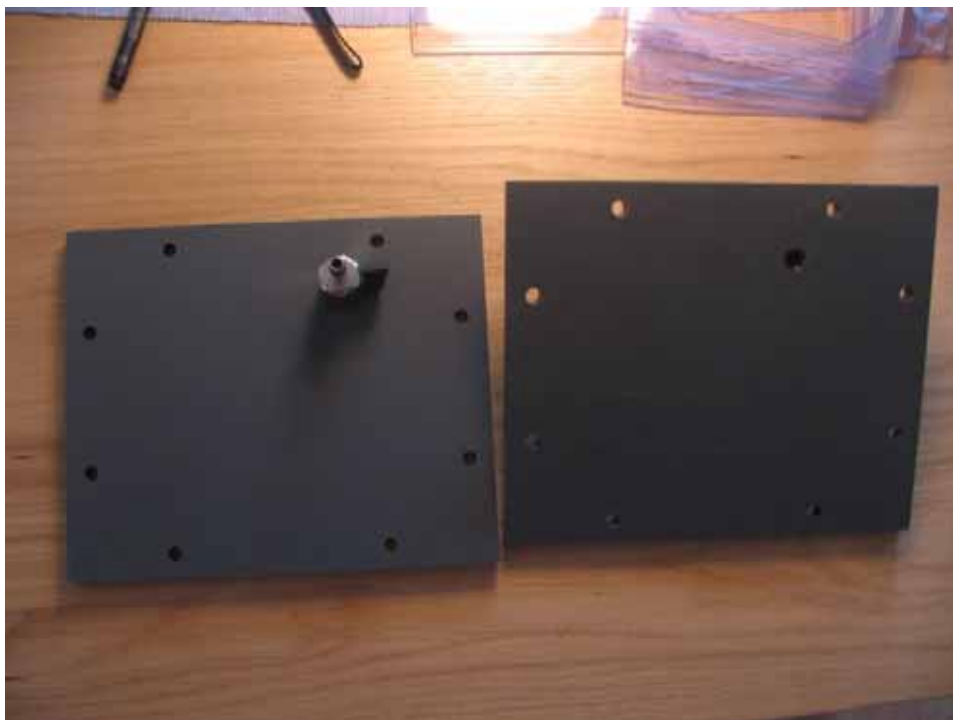
Figure 4. PVC end plates with gas valves attached
