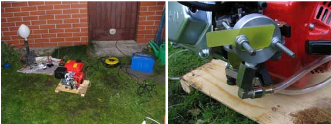
Figure 14. 6.5hp 200cc 4-stroke running on electrolytic gas
