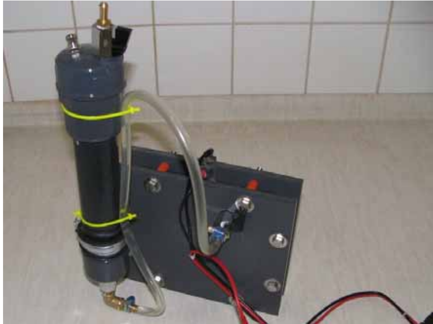
Figure 8. Finished electrolyzer with bubbler
